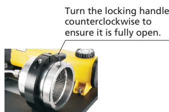
Fig. 3 Unscrew Locking Handle
